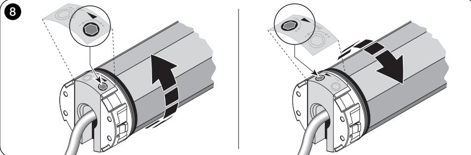
shutter roller rotates, and on the tubular motor locate the adjustment screw marked with the arrow pointing in the same direction as that of rotation (fig. 8).
